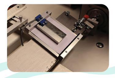
\* Crease stiffness/breaking terms are used interchangeably, they define the point at which a crease being opened transitions from elastic to plastic phase i.e. when permanent change has occurred, in a torque v bending angle test.
