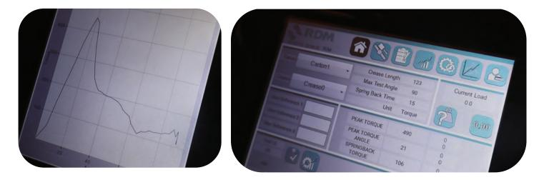
The inside of a TD crease sees more fibre compression as each fibre is squashed into a smaller space which may cause the folding torque to increase as the carton angle approaches 90 degs.
