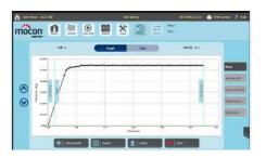
Sequential testing allows a series of tests to be performed on the same samples at different test conditions
