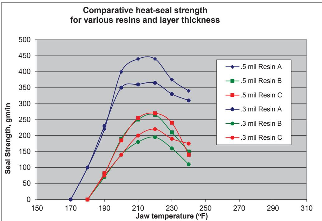
**FIGURE 4.** Representative heat-seal range of heat-sealable substrates with three different melting-point sealant polymers at two different sealant thicknesses.
