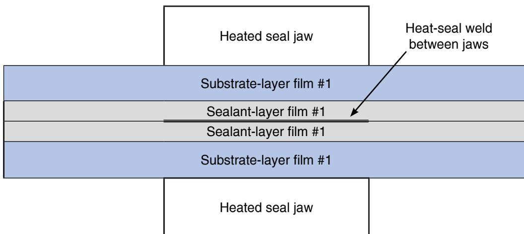
**FIGURE 2.** Heat-sealing two identical heat-sealable film surfaces together with heated sealing jaws. Sealable surfaces melt and weld together due to the jaw temperature, pressure and dwell time of the closed jaws. Jaw temperature is below the melting or distortion temperature of the substrate layer and above the melting point of the sealant layer.
