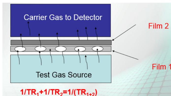
Figure 2. Testing a porous film (Film 1) alongside a nonporous film (Film 2) using the parallel resistance equation.
