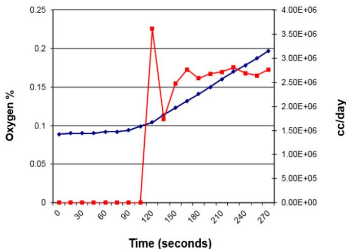
Figure 4. Measuring OTR for perforated films using the Op-Tech O<sub>2</sub> and a test cell.
