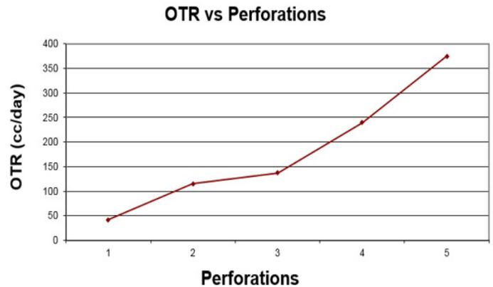
Figure 5. The OTR compared to the number of perforations in the test film.
