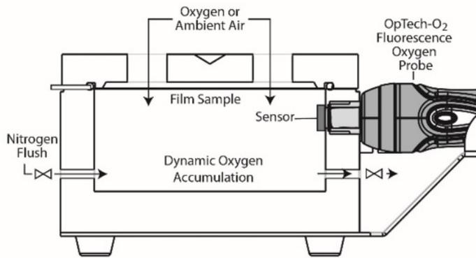
Figure 3. OTR testing with the OpTech-O<sub>2</sub> and a test cell.
