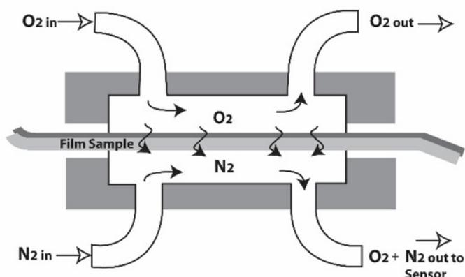
Figure 1. OTR testing using a traditional testing instrument.
