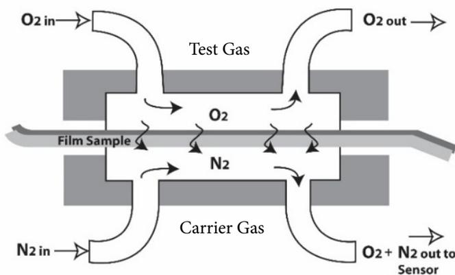
Figure 1. A test cell that uses the isostatic method.
