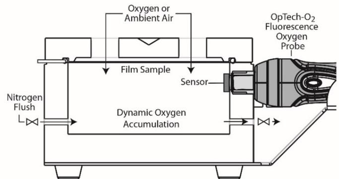
Figure 2. A test cell that uses the dynamic accumulation method.
